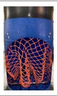
8. Put a bolt through the center bottom hole of the 48" black plastic and the center top hole in the barrel (holes from step 4). Install the remaining 2 bolts to the plastic and the barrel, (use washers on both sides of the bolt). Pull the ends snug to the barrel, mark 1 ½" down from the top of the barrel at the edge of the black plastic. Place the bottom of the plastic on the mark and drill a ¼" hole through the barrel. Install the two end bolts and tighten all 5 bolts.
