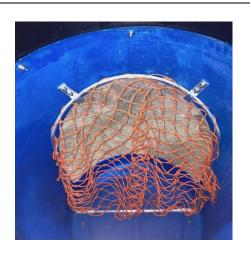
7. Stand the barrel up right and place the net frame in the barrel with the 2 rods sticking out the bottom of the barrel. Pull all net slack down and try to even out the net on the frame. Install and tighten the two net frame brackets and the two hair pins in the net frame on the outside bottom of the barrel.
