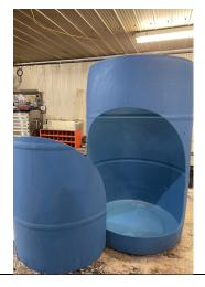
3. Drill all 4-hole marks with a 1/4" drill bit and drill one hole on the inside of the arch to start the jigsaw cut. With the jigsaw cut the bottom horizontal line and all around the arch.
