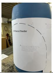
2. Place barrel on a table. Cut along the dotted line on the right side of the paper template and remove that piece to use in step 4. Tape the paper template provided to the barrel. Make sure the feet of the template rest on the table and line up the centerline of the template to a vertical seam in the barrel if possible. Trace the 4 holes at the top, all slots and the bottom line onto the barrel using a marker. Pull off the template
