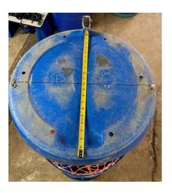
6. Flip barrel upside down, measure along the seam (the same one used to align the template) 10" from the edge (6 o'clock) of the barrel and make a mark. From that mark use a square to make a line perpendicular of the seam and make a mark at 9 o'clock and 3 o'clock. Drill a 9/16" hole through the bottom of the barrel as close to the edge as possible. (At this time drill least 8 more 9/16 holes evenly spaced on the bottom of the barrel for drain holes)
